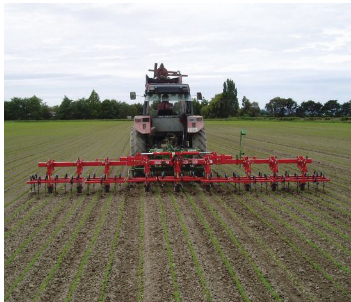
Herbicide alternative: Interrow hoe guided by computer vision.
